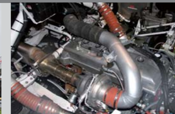
This is the newly developed A09C-TI engine that powered Car 1. This engine, which was deployed while it was still in development, delivered considerably more power than the existing J08C-TI engine.
