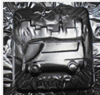
Models of buses and Tokyo SKYTREE were made using a hand press
