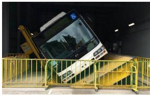
Measuring the most stable incline angle
