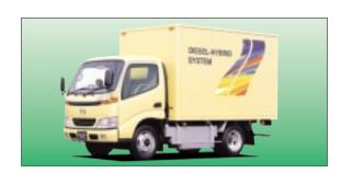
This jointly developed new type of high-fuel economy, clean light-duty diesel-hybrid truck integrates Hino Motors' low-emission diesel engine and Toyota Motor's hybrid system as well as the diesel catalyst system (DPNR). Its development has already advanced to the preparatory stages for an imminent market release in time for the start of supplying low-sulfur light oil.
