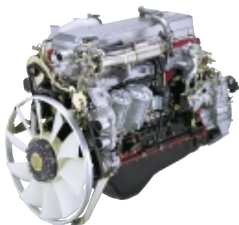
E13C Straight 6-cylinder engine Common-rail fuel injection system Combined EGR Onboard variable nozzle turbo Total displacement: 12.913 L 302 kW (410 PS)
