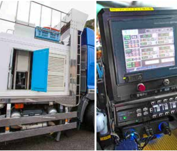
The filtering system was designed to be compact. This monitor enables the driver to check the status of the filtering system.
