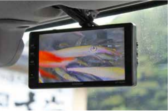
The display above the driver's seat provides a view of the inside of the tank.
