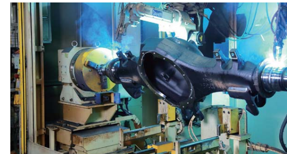
Axle assembly and thick plate welding process that minimizes distortion
