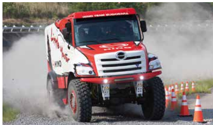
The new Dakar Rally truck has been crafted for improved performance as the team seeks a top overall finish at the Dakar Rally. The vehicle employs a torque converter AT to boost acceleration performance.
