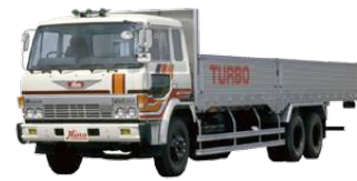
● Super Dolphin Series (Dolphin Turbo 8.8)(1981) This marked the birth of a powerful low-emission vehicle loaded with new ideas and technologies, including the world's first downsized engine using a curved impeller and turbo compressor.
