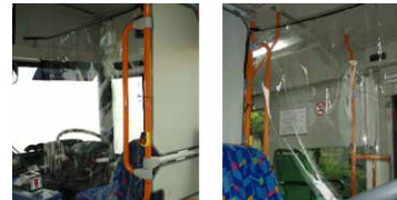
Production of driver's seat protection shield(Bus)
