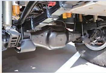
The truck was equipped with new axles for greater ground clearance, and disk brakes that deliver better fade resistance and controllability.
