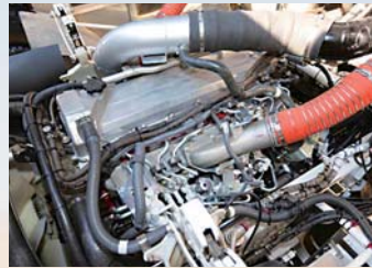
For the first time in Hino's history in the Dakar Rally, this racing truck was powered by an electronically-controlled common rail fuel injection engine.
